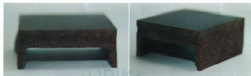
Figure 1 Wood panel samples after 4 weeks of termite test. Left: Front view. A rough edge was due to damage during the cutting process. Right: Side view.
